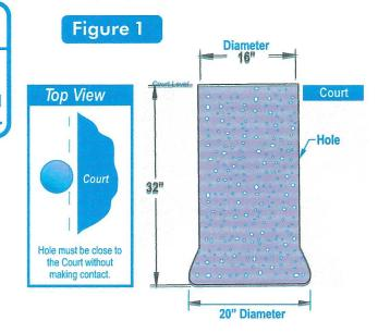
**3.** Place and center a masonry block in the bottom of the hole so there is exactly 16" from the playing surface to the top of the masonry block. See **Figure 2**.
